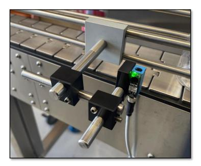
Ensure when setting the sensor that it is set to the flattest part of the container so that the single can reflect back to the sensor, i.e. middle of the container.
