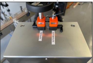
The left scale, when adjusted, will raise the top plate in the BUF, allowing the nozzles to lift higher out of the container. Adjust to enable the BUF to raise far enough that the nozzles lift out of the container and clear the top of the containers by at least 10-15mm.
