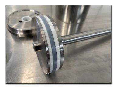
Re-assembly is the reverse of the dismantling procedure. When refitting the Glide-Ring Seal and its O-ring to the piston head, particular care should be taken. The seal should be eased into place by hand - do not use screwdrivers or other sharp implements which will damage the seal. It is important that the seal is installed square on the piston head for its full circumference.
