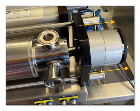
The complete assembly can be now removed to a bench or sink where the component parts will simply pull apart for cleaning.
