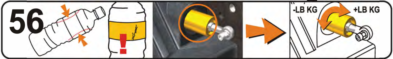
ADJUSTING PRESSURE FOR FRAGILE CONTAINERS
