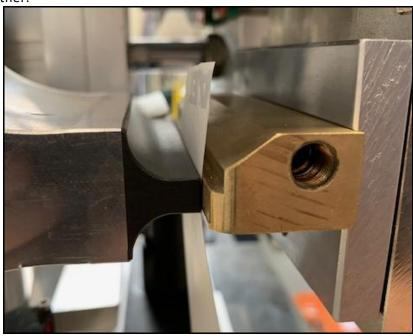
Test by cutting the end of a tube and seeing if you can place the flattened tube between the moulds. A correct adjustment will show to have some drag on the tube when sliding between the moulds.
