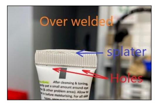
Over-welding will show as very rounded outer edges, splatter to the top of the tube and/or holes in the bottom seam.
