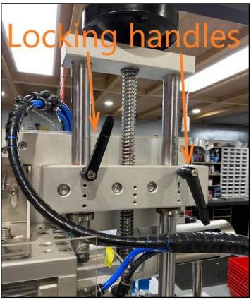
Once unlocked: wind the large handle wheel on top of the machine left or right to adjust the height of the welding mould and trimmer to suit the desired height.
