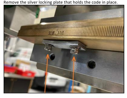
Using a flat blade screwdriver push out the letters/numbers from within the hole where locking plate was removed.
