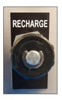
The product cylinder recharge rate should be adjusted so that the cylinder is recharged as quickly as possible, but with adequate time for exchanging the filled container under the nozzle with an empty one.
