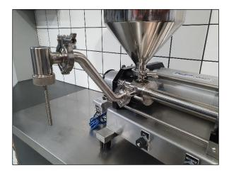
Ensure gooseneck plug is installed and finger tight – this is removable for cleaning purposes.
