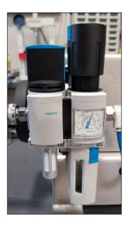
Connect the main compressed air supply line via a NITO or similar connection fitting on the Air Pressure Regulator/Filter. Located on the rear corner of the machine. Ensure that the Hand Valve is turned to EXH (off position).
