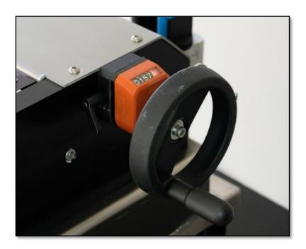
The handwheel at the side of the machine controls the fill volume, and the digital scale gives you the ability to fine-tune the fill volume easily, and to be able to return to a noted volume without having to re-calibrate the fill volume.
