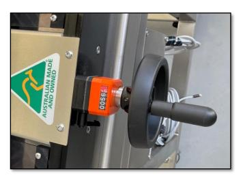
Ensure to lock off the handle once adjusted to limit any possible movement whilst the machine is in operation.
